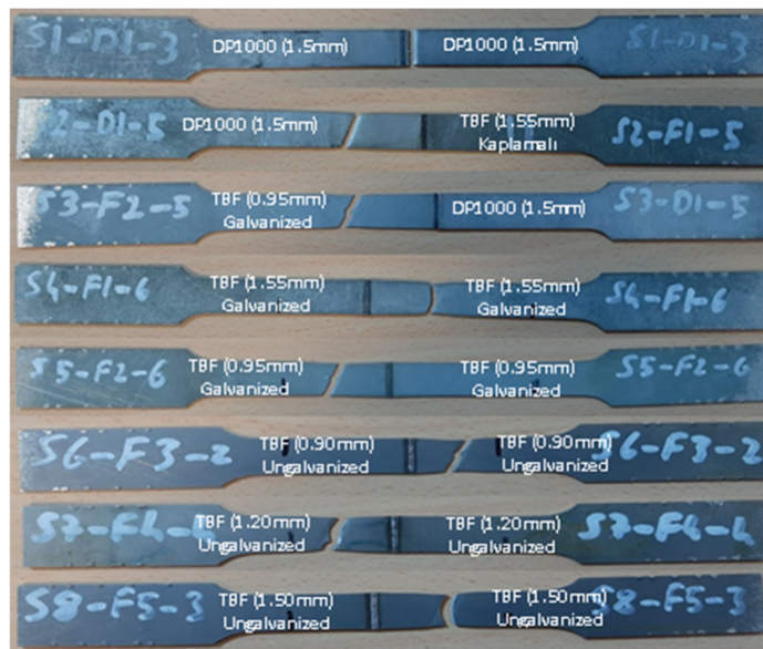
Figure 3. Fracture regions of the laser welded samples after tensile test.
