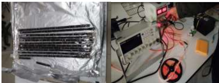
Figure 5. The images of sliced mono-c silicon for luminescent plates of 50x50 cm 2 size and strip LEDs to be used as loads.
