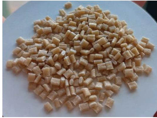
Figure 2. Produced HDPE/Celestite composite granules
