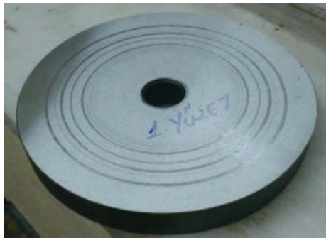
Figure 3. AISI 8620 case hardening steel counter face disc
