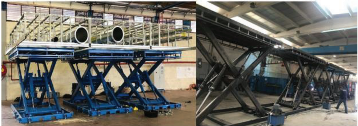
Figure 9. Simultaneous Scissor Platform Prototype
