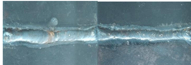
Figure 7: Best weld from manual welding
