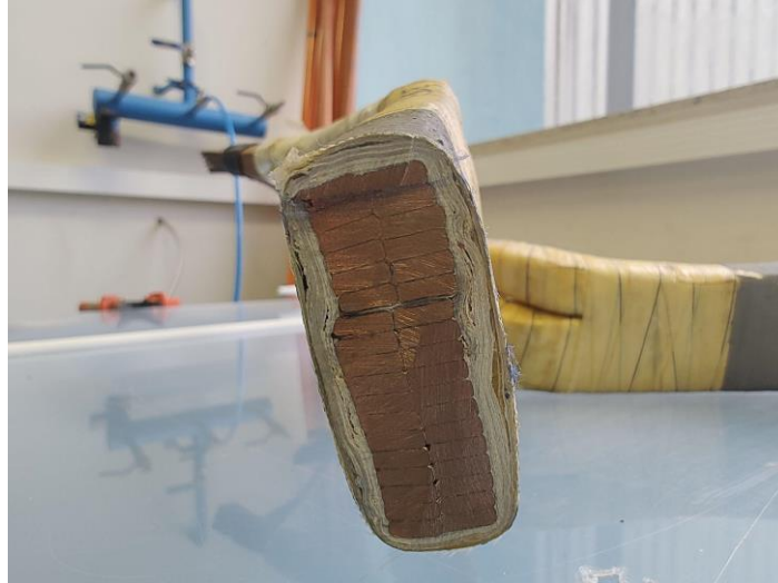
Fig.02: The defective stator bar cross section.
