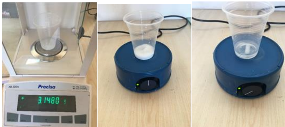
Figure 3. Images of weight of NaOH in distilled water, after addition ZnO in solution (before mixing of solution), and then one hour mixing of solution.
