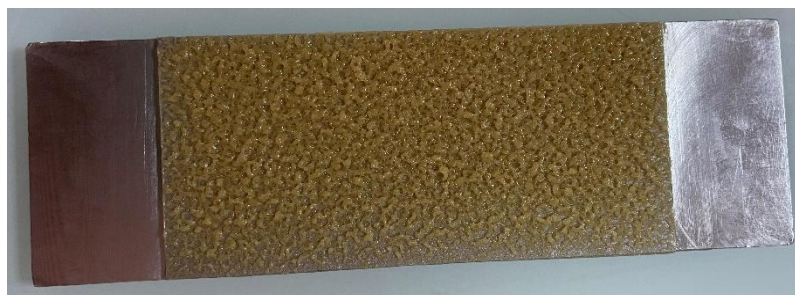
Figure 3: Appearance of PAO Based CSX After Water Spray-Off resistance Test
