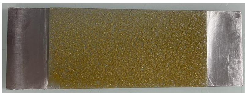
Figure 4: Appearance of Mineral Oil Based CSX After Water Spray-Off resistance Test
