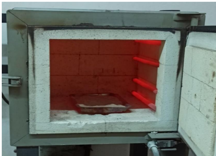
Figure 1. The calcination process of the starting raw material at 900^\circ\text{C} .
