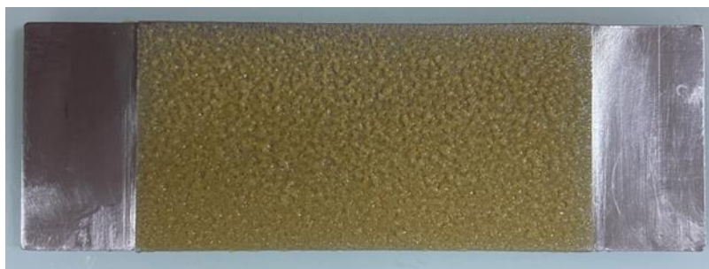
Figure 2: Appearance of Ester Based CSX After Water Spray-Off resistance Test
