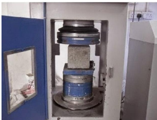
Broken specimen when the load is applied
