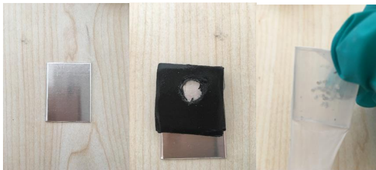
Figure 2. Anode part of test battery, gaskets and the air-contact face is covered with commercial teflon tape film.
