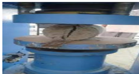
Compressive strength testing machine showing cylinder subjected to loading
