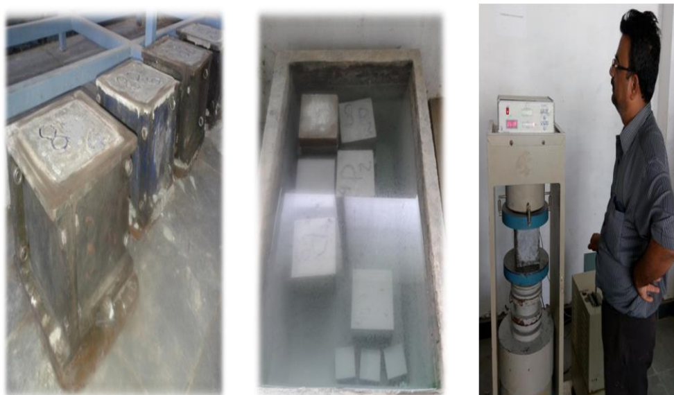
Fig 4: CASTING, CURING AND TESTING OF CUBES
