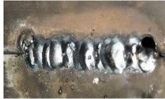
Figure 5: Worst Weld from manual welding
