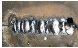
Figure 6: Worst Weld from manual welding
