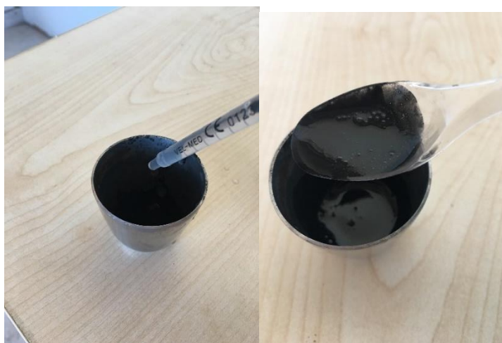
Figure 1. PVA adhesive in the syringe is added to the container with AC and MnO 2 .
