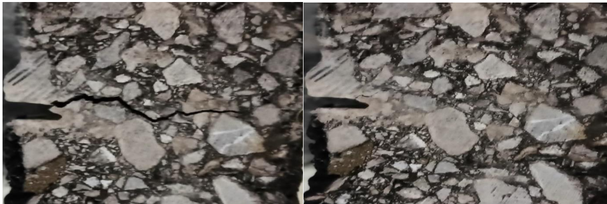
Figure 4: Healing of crack after microwave heating
