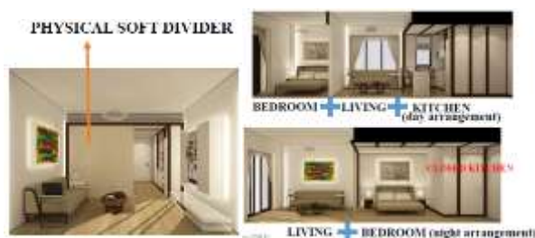
Figure 2. Horizontal overlapping of spaces; sliding light panels are used to create sub-spaces
