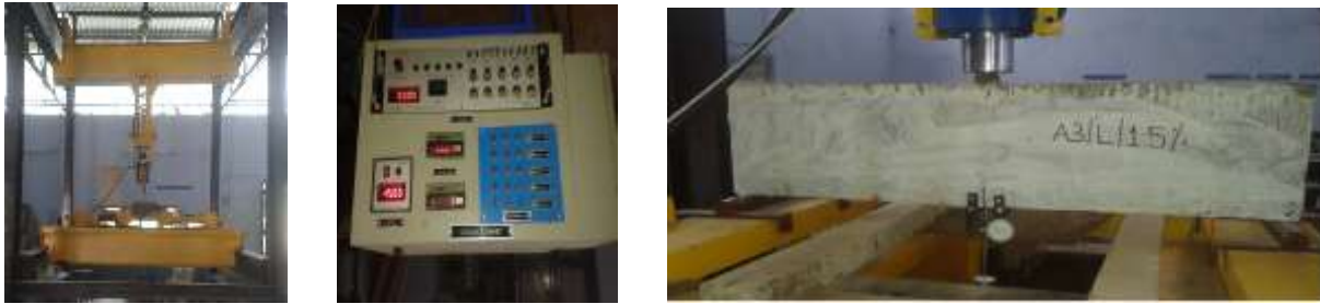
Loading Frame Test setup Used for Testing of Beams
