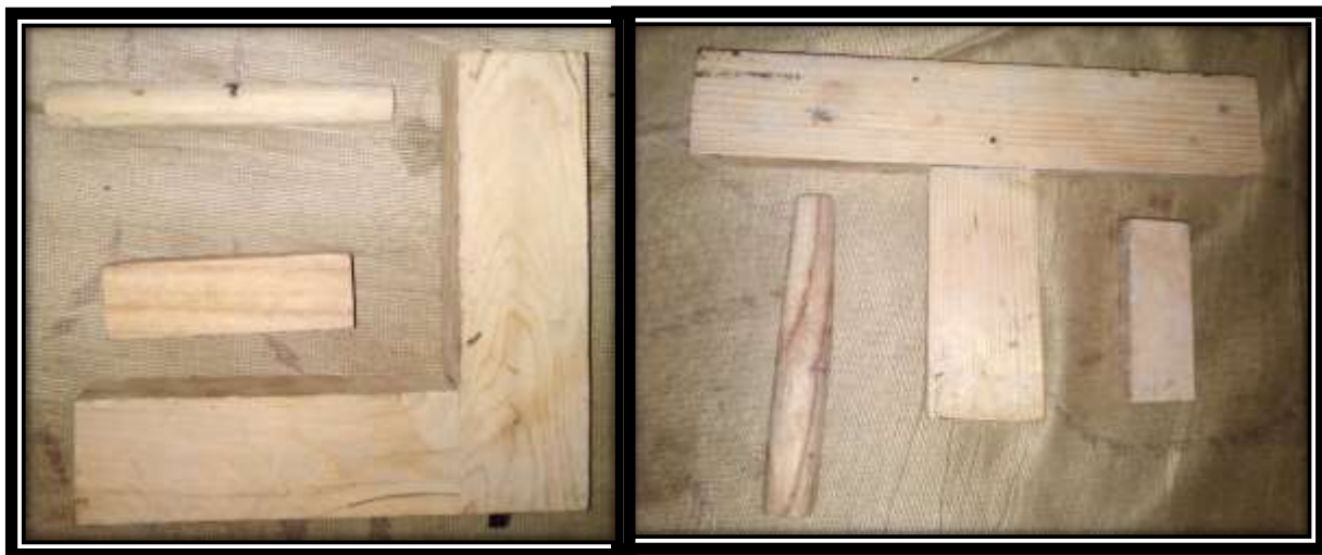
Figure 3.3a pattern for T & L shape casting
