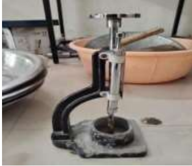
Fig:6-Penetration test Test
