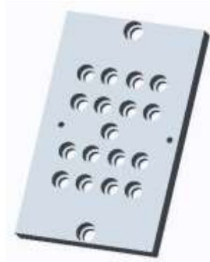
Figure 5: Ejector Retaining Plate 3D Model
